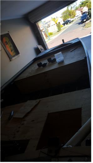
The front was to be raised to just under the level of the gunnel. This was scary as we were not sure how stable the boat would be. The fuel tank was to be moved under the front deck to help with balance. I also wanted a lean bar so I can drive in a standing position and something to grab when I am on the dance platform (front deck) and the bow wave from that 40-foot Riviera sneaks up on me. I also wanted rod storage for 9-foot rods.
